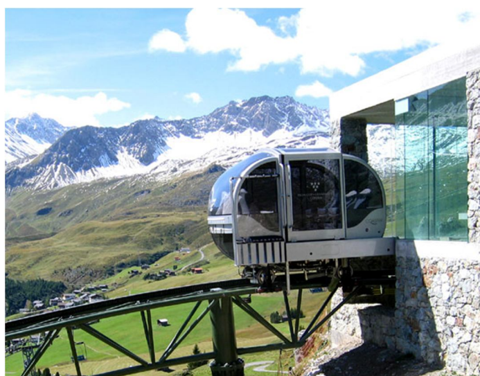
Slika 2: PRT (Personal Rapid Transit) sistem Coaster u Arosi, Švajcarska (izvor: www.coaster.at )
