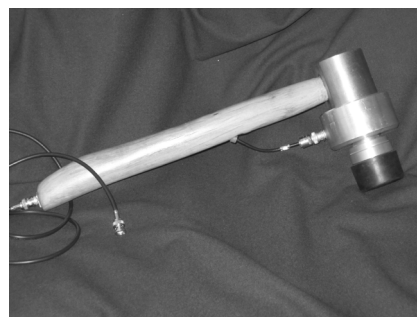
Fig. 7. Impact excitation by means of modal testing hammer
