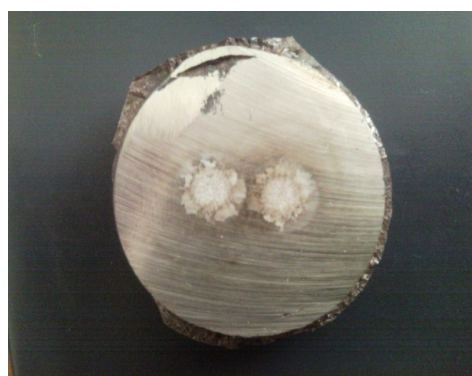
Fig.6. Spectrum analysis test specimen that burned from its two different zones.
