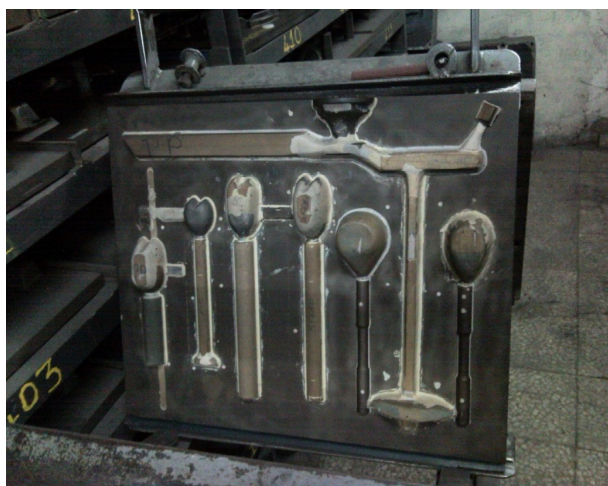
Fig.1. A model for sand moulding
